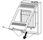
Figure 10 - Removing Front Panel Of Heater
